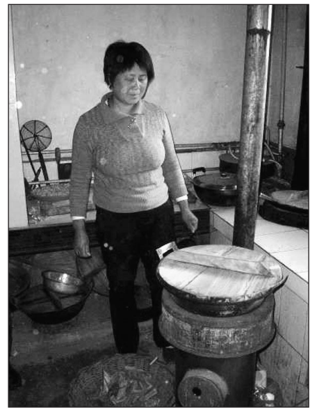
Figure 2 Luoyang gasifier stove installed in kitchen (photo: CEIDH)
