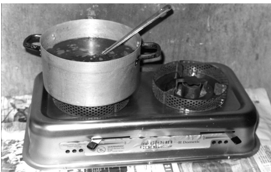
Figure 2 CleanCook stove after three years of constant use (photo: Project Gaia)
