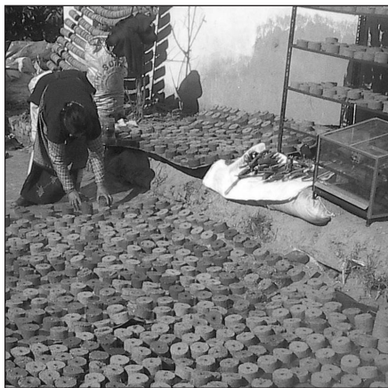
Figure 2 Environmentally friendly drying of briquettes (photo: FoST)
