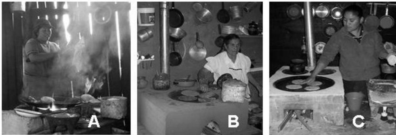
Figure 1. Traditional open fire (A), mud-cement Patsari (B), and brick Patsari (C) (Photo: M. Johnson)
