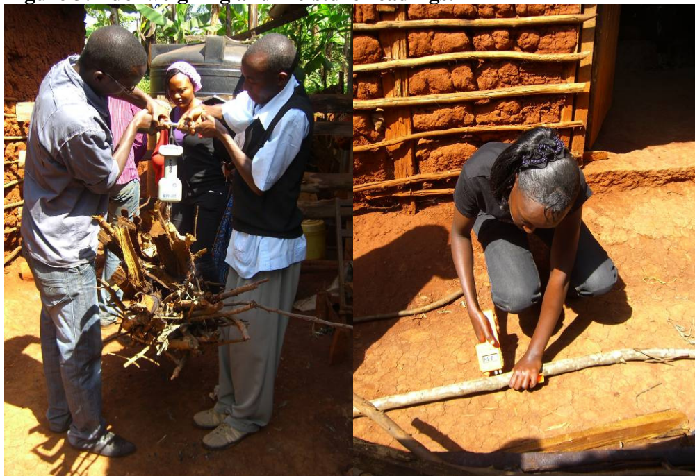
Figure 3: Fuel weighing and moisture readings.
