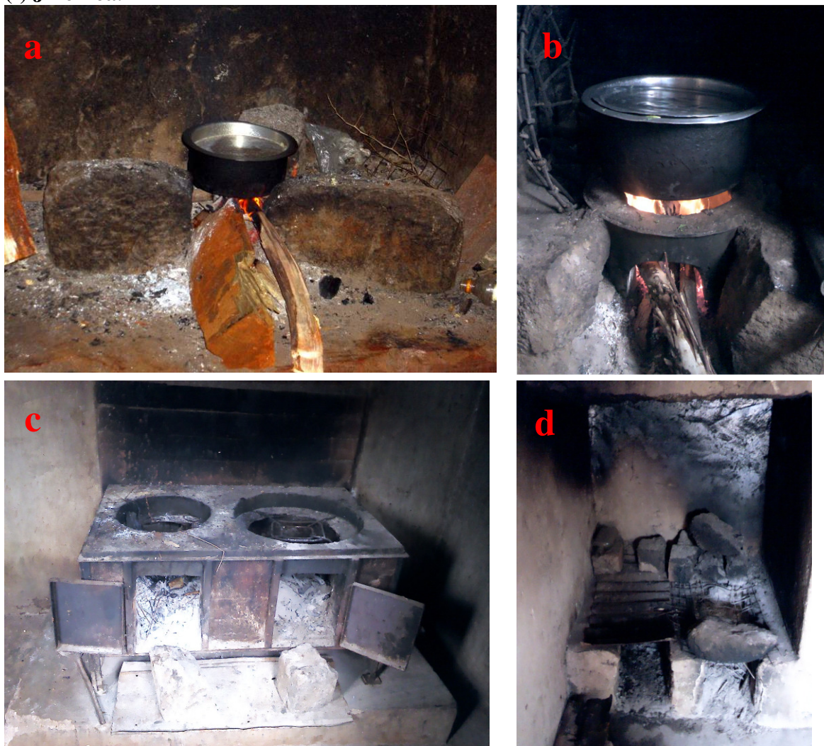
Figure 2: Stove photos: (a) three-stone fire, (b) Jiko Kisasa, (c-e) other baseline stoves, and (f) Jiko Poa.
